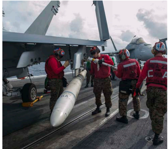
Marines assigned to the Thunderbolts of Marine Fighter Attack Squadron (VMFA) 251 remove a training AGM-88 HARM from an F/A-18C Hornet on the flight deck of the Nimitz-class aircraft carrier USS Theodore Roosevelt (CVN 71).
